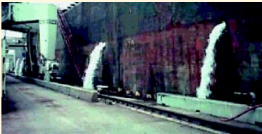
To stabilize the empty freighters, large amounts of water are carried in ballast. Small planktonic organisms--sometimes even fish--are pumped in with the ballast water and may survive the ocean voyage.
